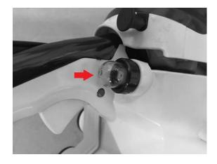
Pull the choke lever. It will close and the throttle will be moved to the starting position
